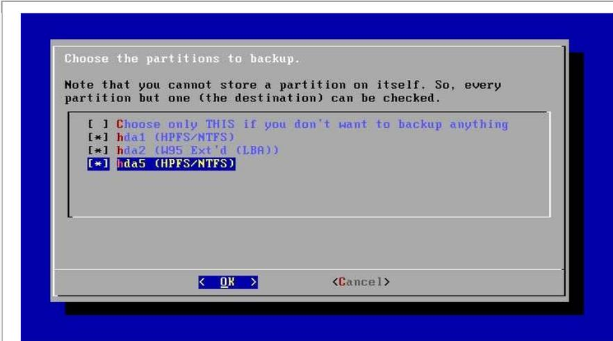
All connected hard disk drives, USB mass storage devices included, will be scanned and all available partitions should be enumerated here, with either a NTFS label, or first found directories.
