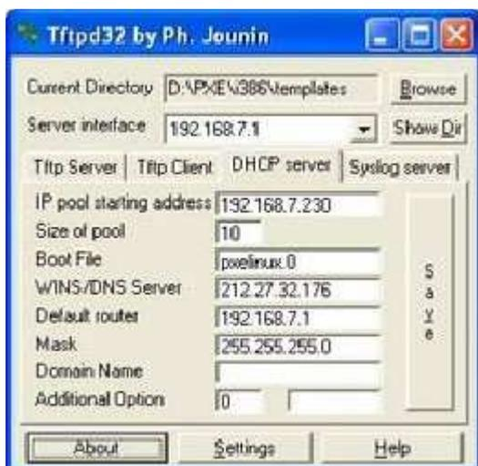
Configure your **DHCP Server** here. Booting with PXE is not possible unless you define it. A common network configuration is to have addresses like 192.168.0.x with 192.168.0.1 as the router (often a workstation connected both to the internet, both to the LAN, and sharing the internet connection on the LAN).
